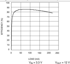
Figure 21. Efficiency vs Load Current - Y Option
