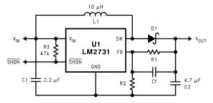
Figure 26. Basic Application Circuit
