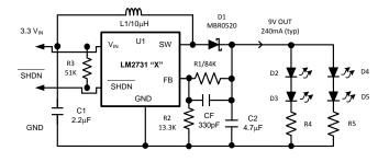
Figure 38. VIN = 3.3 V, VOUT = 9 V at 240 mA
