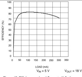
Figure 17. Efficiency vs Load Current - X Option
