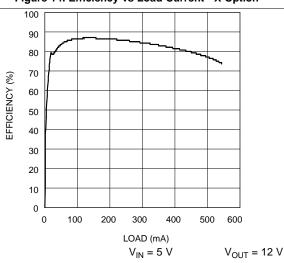
Figure 16. Efficiency vs Load Current - X Option
