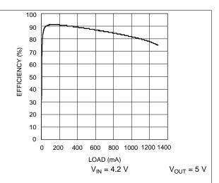
Figure 19. Efficiency vs Load Current - Y Option
