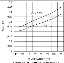
Figure 10. R<sub>DS</sub>(ON) vs Temperature
