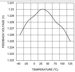
Figure 9. Feedback Voltage vs Temperature
