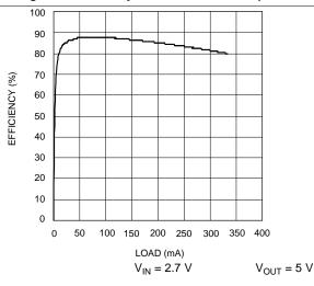
Figure 18. Efficiency vs Load Current - Y Option
