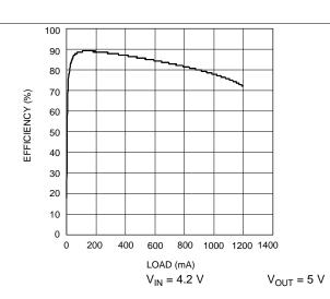
Figure 14. Efficiency vs Load Current - X Option
