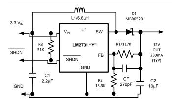
Figure 36. VIN = 3.3 V, VOUT = 12 V at 230 mA
