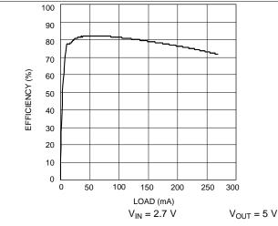
Figure 13. Efficiency vs Load Current - X Option
