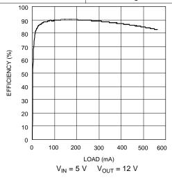
Figure 23. Efficiency vs Load Current - Y Option
