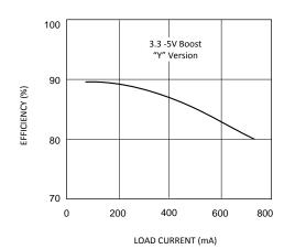
Figure 35. Efficiency vs Load Current
