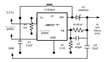
Figure 34. VIN = 3.3 V, VOUT = 5 V at 700 mA
