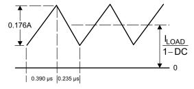
Figure 27. 10 µH Inductor Current, 5 V-12 V Boost (LM2731X)
