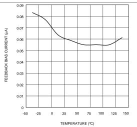
Figure 8. Feedback Bias Current vs Temperature
