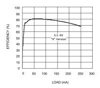
Figure 39. Efficiency vs Load Current
