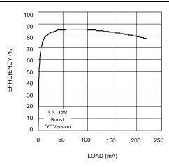
Figure 37. Efficiency vs Load Current
