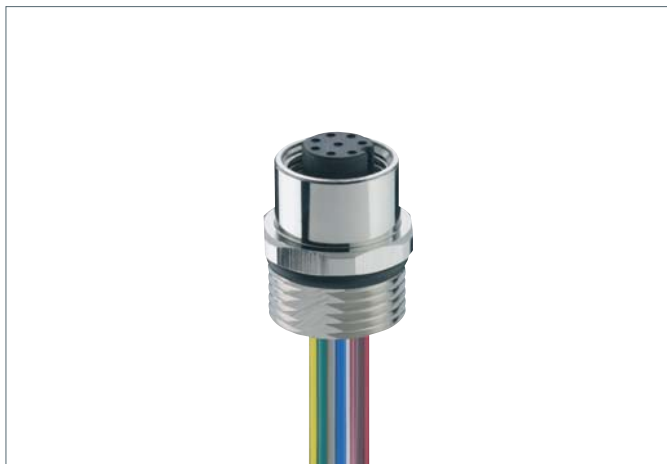
M12 panel mount connector, female, A-coded, IP67, for front mounting, thread M16, with stranded wires
