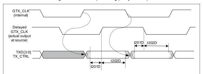
Figure 50: RGMII Output Timing (Delayed Mode)
