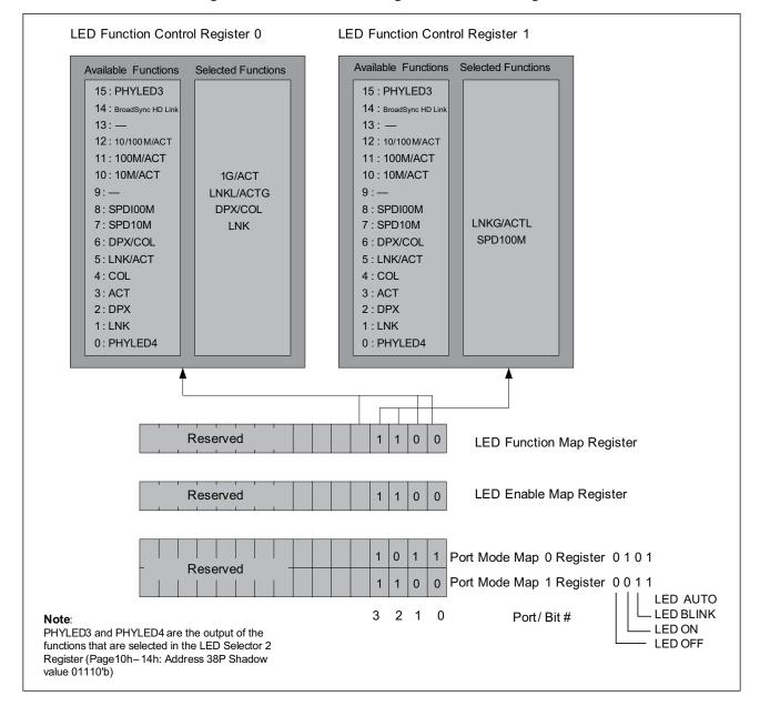
Figure 44: LED Interface Register Structure Diagram
