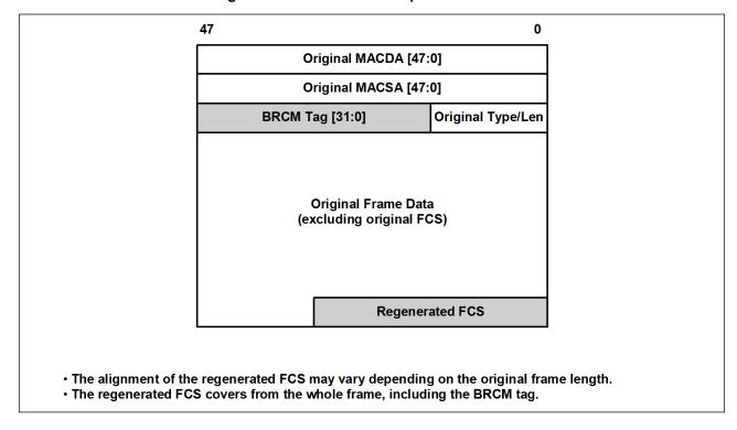
Figure 12: IMP Packet Encapsulation Format
