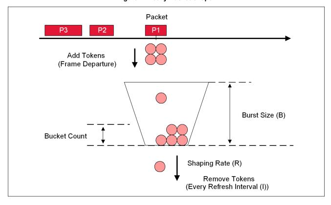
Figure 4: Leaky Bucket Shaper
