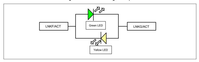
Figure 46: Dual LED Usage Example
