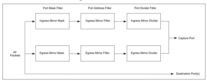
Figure 10: Mirror Filter Flow
