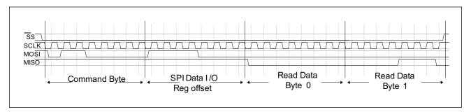
Figure 23: Normal Read Mode to Obtain the Register Content
