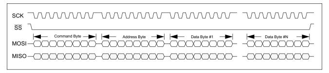
Figure 14: SPI Serial Interface Write Operation
