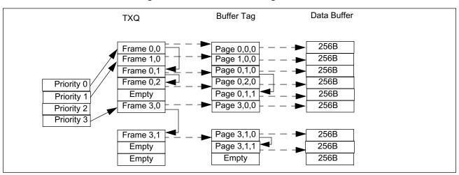
Figure 13: TXQ and Buffer Tag Structure
