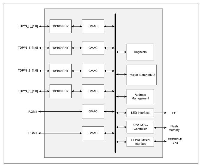
Figure 1: BCM53106S Functional Block Diagram
