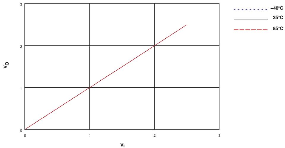
**Figure 1.  $V_O$  vs  $V_I$ ,  $V_{CC} = 2.5\text{ V}$**
