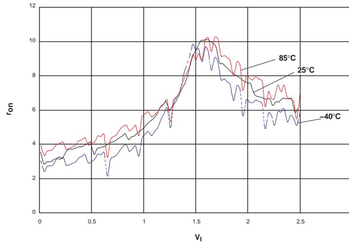
**Figure 4.**  $r_{on}$  vs  $V_I$ ,  $V_{CC} = 2.5$  V
