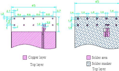
Tolerances unless otherwise specified ±0.1mm t,w=Unique dimensioning according to your PCB.
