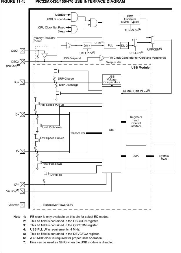
FIGURE 11-1: PIC32MX430/450/470 USB INTERFACE DIAGRAM
