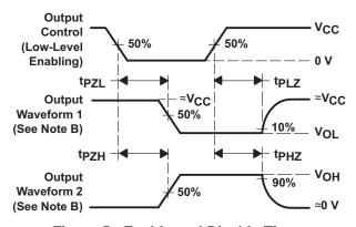
Figure 5. Enable and Disable Times for 3-State Outputs
