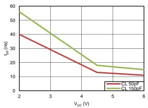
Figure 1. Propagation Delay
