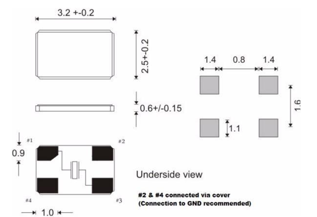
Holder Style Mode Adjustment Tolerance Temperature Stability Operating Temp. Range Load Capacitance ESR Drive Level Static Capacitance (C0) Dynamic Capacitance (C1) Ageing Marking 3X25X06 4-Pad Fundamental ± 10PPM at 25°C ± 20 PPM -40°C to +85°C 9 pF 80 Ohm 0.1 mW As Typ. pF As Typ. pF As Typ. fF +/-3ppm/year AEL16 WWYY
