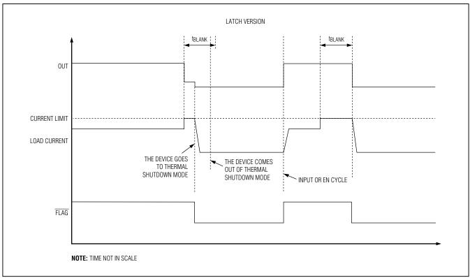
Figure 2. Latch-Off Fault Diagram
