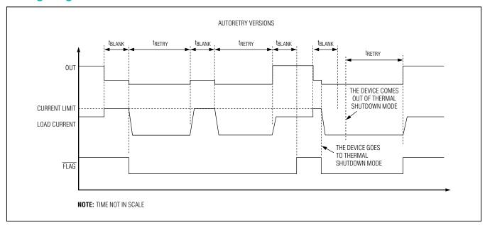
Figure 1. Autoretry Fault Diagram
