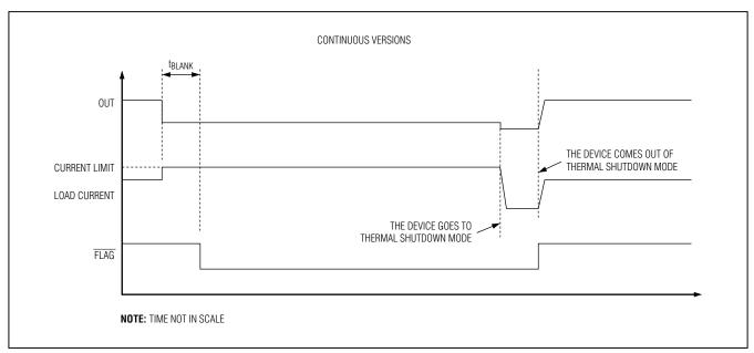
Figure 3. Continuous Fault Diagram
