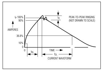
Figure 5b. Human Body Current Waveform
