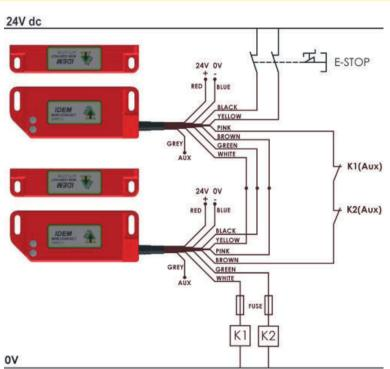
Two switches connected in series to give dual circuit safety outputs to machine contactors.
