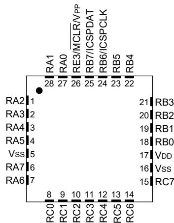
**Note:** It is recommended that the exposed bottom pad be connected to  $V_{SS}$ , however it must not be the only  $V_{SS}$  connection to the device.
