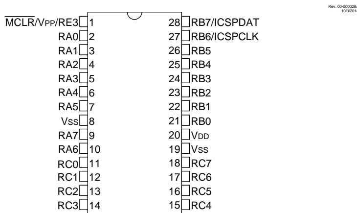
**Figure 2. 28-pin , VQFN**
