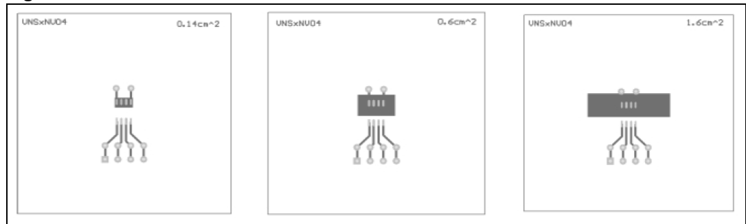
Figure 37. SO-8 PC board (1)
