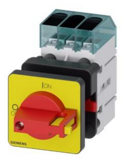
Load disconnector 3LD3, lu 16 A Main switch 3-pole Rated operating capacity at AC-23 A at 400V 7.5kW Front plate mounting Basic switch with Central hole mounting 22.5mm Toggle drive red / yellow 48x48 mm
