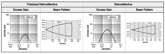
Fixed-field focus and spot sizes are typical. Performance based on use of 90% reflectance white test card.\*
