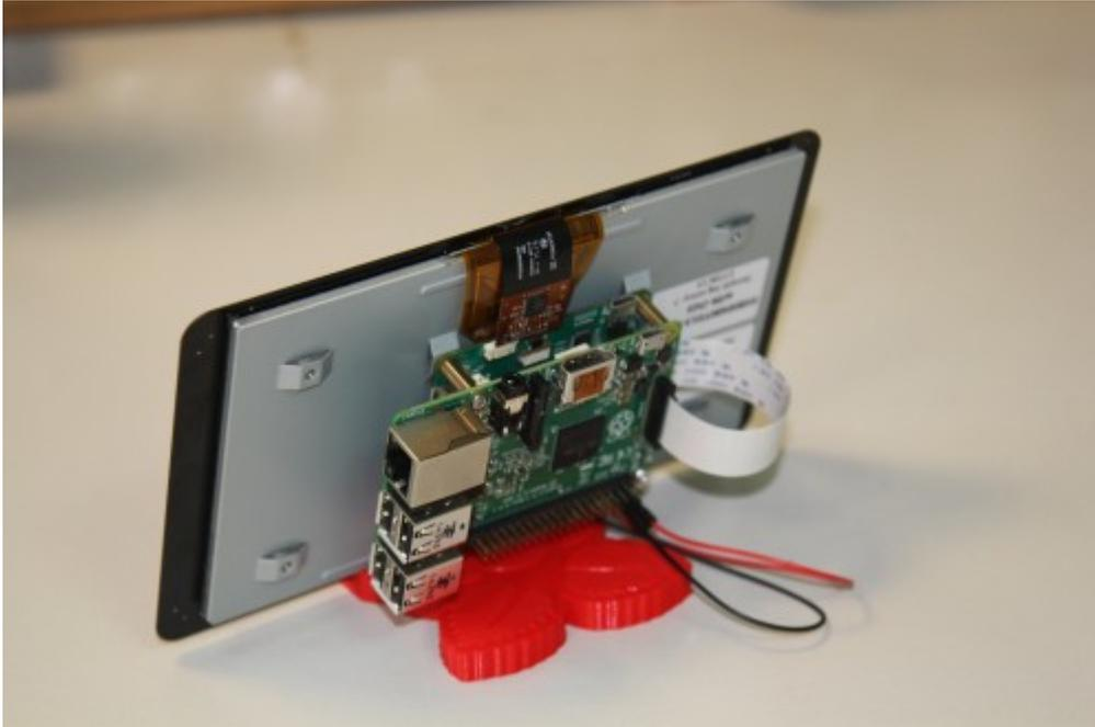
The 15-way FPC connector should already be plugged into the display conversion board with the silvered contacts face-up. You can then plug the connector into the Raspberry Pi with the silvered connectors inboard (facing towards the USB connectors).
