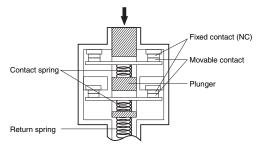
Conforms to EN60947-5-1 Direct Opening Operation  $\bigcirc$
