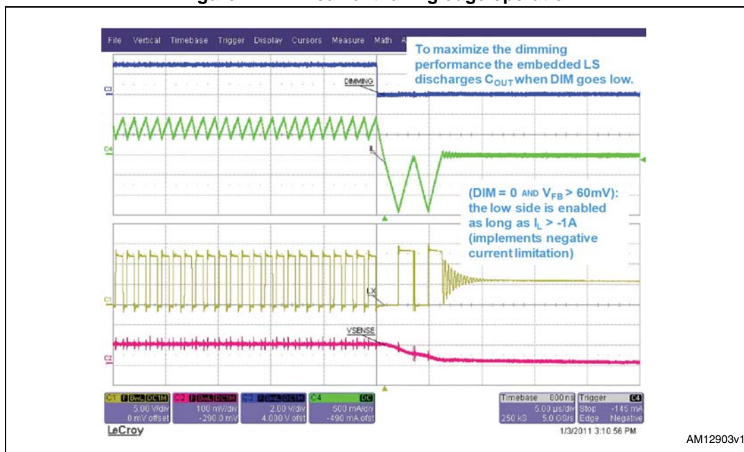
Figure 12. LED current falling edge operation
