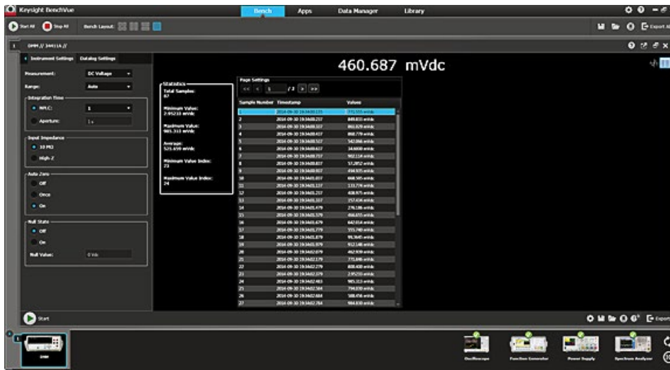
Figure 2. BenchVue enables control of your DMM to data log and visualize measurements in a wide array of display options.
