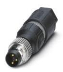
Sensor/actuator connector, Universal, 3-position, Plug straight M8, A-coded, Insulation displacement connection, knurl material: Nickel-plated brass, external cable diameter 2.5 mm ... 5 mm
