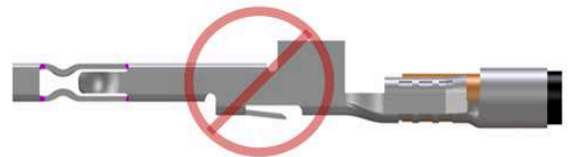
Collapsed Locking Tab
