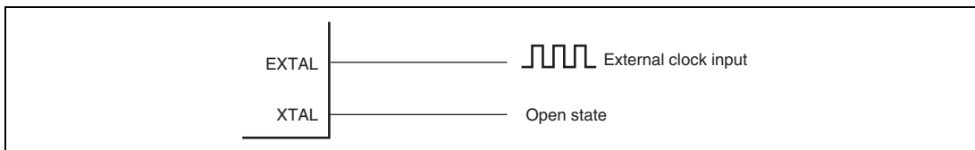
Figure 4.4 Example of External Clock Connection
