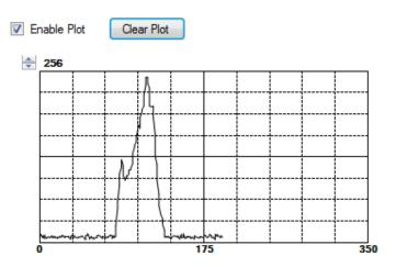
The **Enable Plot** checkbox activates the plotting function. Data will only be plotted when this box is checked.
