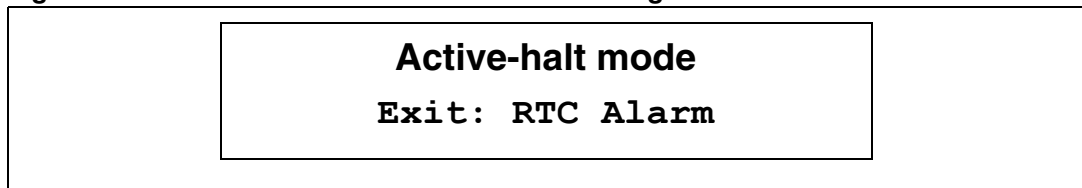
Figure 29. Exit from Active-halt with alarm message
