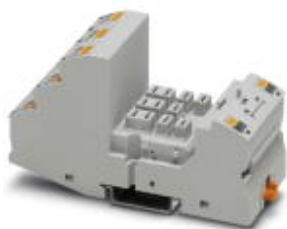
RIF-4... relay base, for high-power relay with 2 or 3 PDTs or 3 N/O contacts, Push-in connection, plug-in option for input/suppressor modules, for mounting on NS 35/7,5
