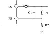
Figure 1. Feedback Divider Network
