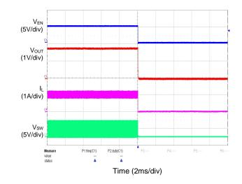
Enable Turn Off Characteristic (Iout = 1A)
