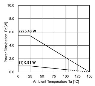
Figure 34. Power Dissipation Graph (TO252-5)
