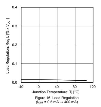
Unless otherwise specified,  $V_{IN}$  = 13.5 V,  $V_{OUT}$  setting = 5 V,  $V_{EN}$  = 5 V,  $R_1$  = 120 k $\Omega$ ,  $R_2$  = 803 k $\Omega$ ,  $R_3$  = +25 °C
