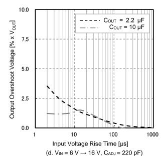
Figure 18. Line Transient Response  $(V_{IN} = 6 \text{ V} \rightarrow 16 \text{ V})$
