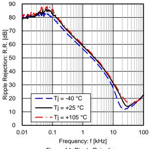
Figure 14. Ripple Rejection (ein = 1 Vrms, I<sub>OUT</sub> = 100 mA)
