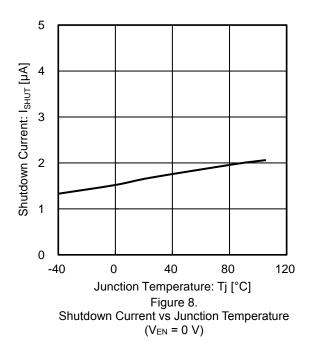
Unless otherwise specified,  $V_{IN}$  = 13.5 V,  $V_{OUT}$  setting = 5 V,  $V_{EN}$  = 5 V,  $R_1$  = 120 k $\Omega$ ,  $R_2$  = 803 k $\Omega$
