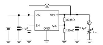
Measurement Setup for Figure 9
