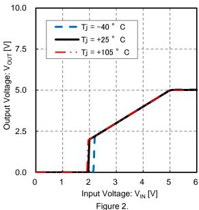
Output Voltage vs Input Voltage -Enlarged view
