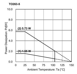
Figure 36. Power Dissipation Graph (TO263-5)
