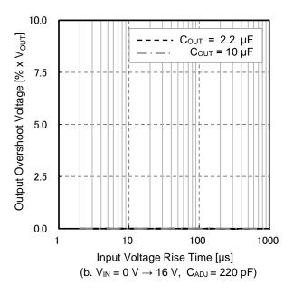
Figure 17. Line Transient Response  $(V_{IN} = 0 \text{ V} \rightarrow 16 \text{ V})$
