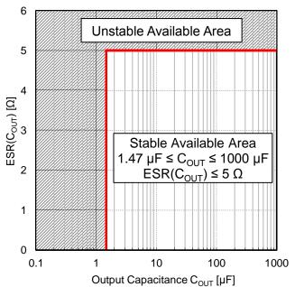
Figure 23. Output Capacitance  $C_{OUT}$ , ESR Stable Available Area (-40 °C  $\leq$  Tj  $\leq$  +105 °C, 6 V  $\leq$  V<sub>IN</sub>  $\leq$  42 V, V<sub>EN</sub> = 5 V, I<sub>OUT</sub> = 0 mA to 500 mA)
