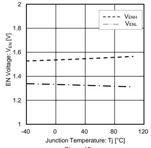
Figure 12. EN Input Voltage vs Junction Temperature
