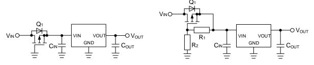
Figure 31. Protection against Reverse Polarity 2
