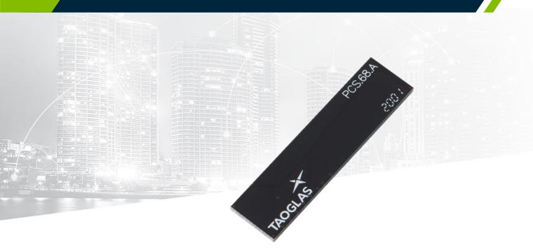
The Taoglas Reach Series PCS.68.A is a revolutionary 5G/4G, low profile, small footprint, patent pending, SMD mount PCB wide-band antenna. The PCS.68.A has been designed to cover all 5G and 4G bands, including all sub-6GHz deployments across the 600MHz to 6000MHz spectrum in a very small footprint of just 42 x 10mm. It also covers 3G/2G bands to allow for fall-back when 5G/4G is not available. The low profile size of just 1.5mm in height allows for installation where height is at a premium.
