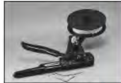
Contact Crimp Hand Tool (300 Contact Reel)
