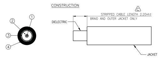
NOTE: JACKET STRIP OD DEFORMED MUST BE THAN LESS Ø3.30mm AFTER CUT OFF.
