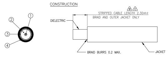
NOTE: JACKET STRIP OD DEFORMED MUST BE THAN LESS \$2.75mm AFTER CUT OFF.
