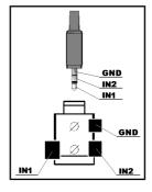
The socket can interface standard 3.5 mm phone connector (also known stereo plug or audio plug).
