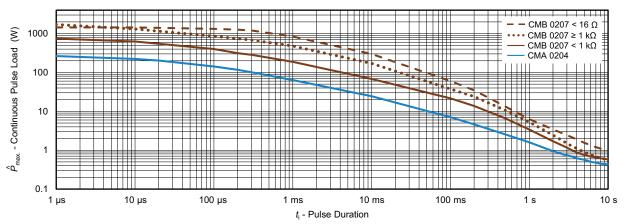
Maximum pulse load, continuous pulse; applicable if  $\overline{P} \le P$  ( $\vartheta_{amb}$ ) and  $\hat{U} \le 4$  kV (CMB); or  $\hat{U} \le 2$  kV (CMA); for permissible resistance change  $\pm$  (0.5 % R + 0.01  $\Omega$ )
