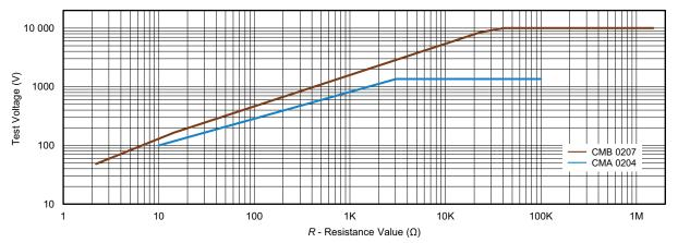
Pulse load rating in accordance with IEC 60115-1, clause 4.27; 10  $\mu$ s / 700  $\mu$ s; 10 pulses at 1 minute intervals; for permissible resistance change  $\pm$  (0.5 % R + 0.05  $\Omega$ )
