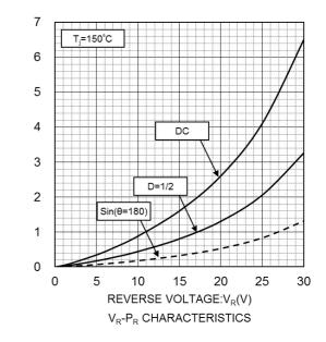
REVERSE POWER DISSIPATION:P<sub>R</sub>(mW)
