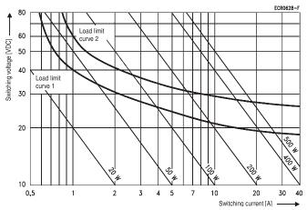
Load limit curve 1: arc extinguishes during transit time (CO contact).
