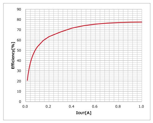
Figure 11. Efficiency vs Load Current
