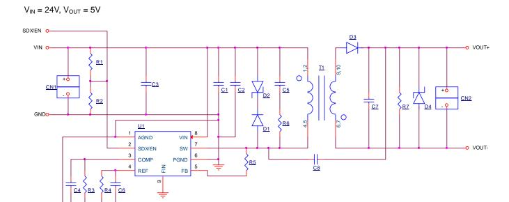
Figure 4. BD7F100EFJ-EVK-001 Circuit Diagram
