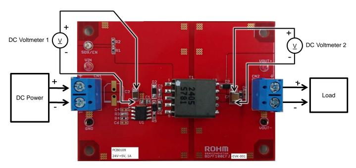
Figure 3. Connection Diagram
