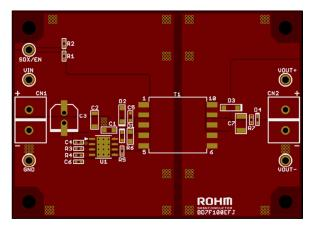
Figure 5. Top Silk Screen and Layout (Top View)
