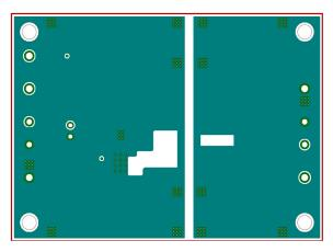
Figure 8. Middle Layer1 Layout (Top View)
