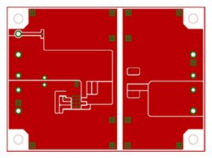
Figure 7. Top Side Layout (Top View)
