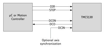
Figure 19.4 Full signal interconnection for DcStep
