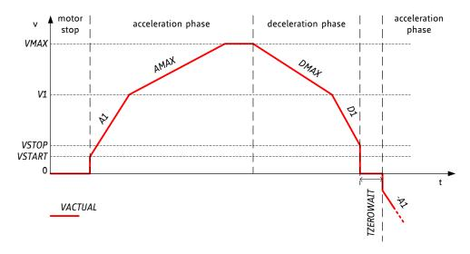
Figure 14.1 Ramp generator velocity trace showing consequent move in negative direction
