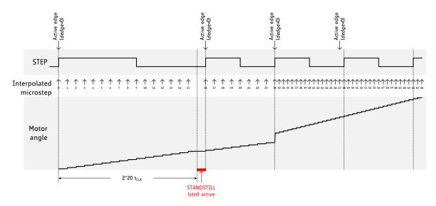
Figure 17.2 MicroPlyer microstep interpolation with rising STEP frequency (Example: 16 to 256)
