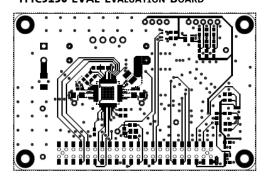
The TMC5130-EVAL is part TRINAMICs universal evaluation board system which provides a convenient handling of the hardware as well as a user-friendly software tool evaluation. The TMC5130 evaluation board system consists of three parts: STARTRAMPE board), (base ESELSBRÜCKE (connector hoard including several test points), and TMC5130-EVAL.
