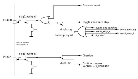
Figure 18.2 DIAG outputs with SD\_MODE=0
