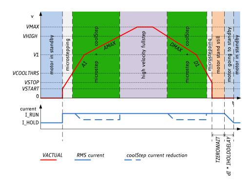
Figure 14.3 Ramp generator velocity dependent motor control
