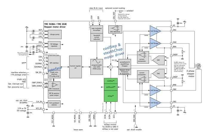
Figure 1.2 TMC5130A STEP/DIR application diagram
