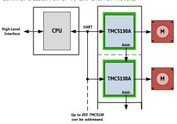
An application with 2 stepper motors is shown. Additionally, the ABN Encoder interface and two reference switches can be used for each motor. A single CPU controls the whole system. The CPU-board and the controller / driver boards are highly economical and space saving.
