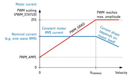
Figure 7.5 Velocity based PWM scaling (pwm autoscale=0)
