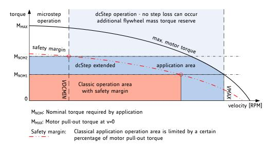
Figure 19.1 DcStep extended application operation area
