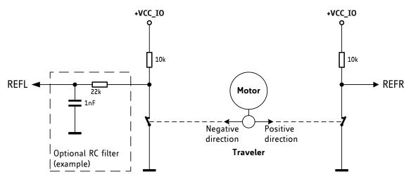
Figure 14.4 Using reference switches (example)
