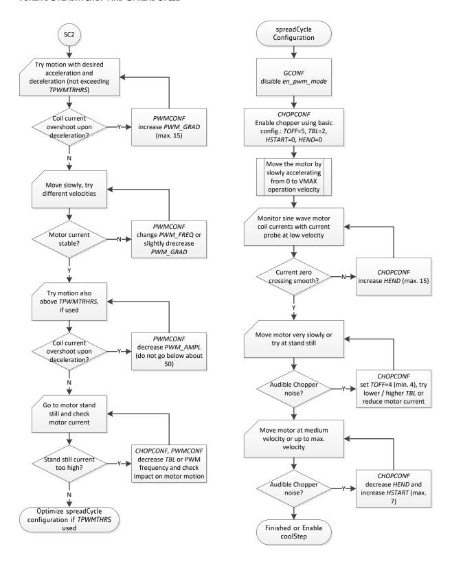
Figure 24.2 Tuning StealthChop and SpreadCycle
