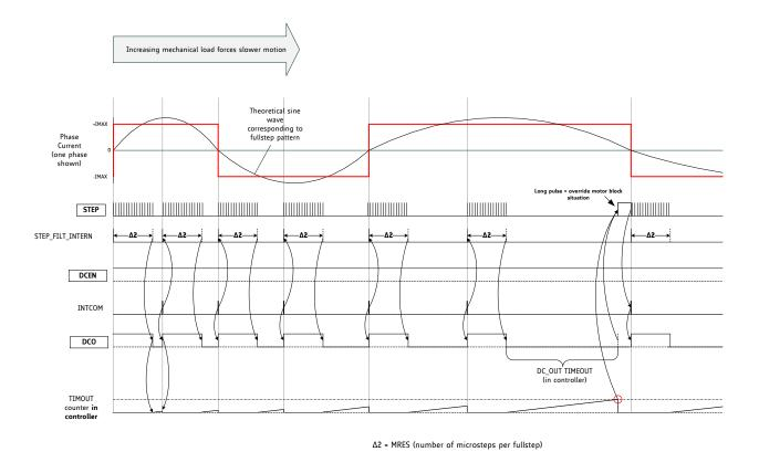
Figure 19.5 DCO Interface to motion controller - step generator stops when DCO is asserted
