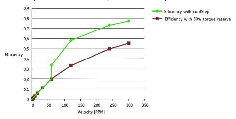
Figure 1.4 Energy efficiency with CoolStep (example)
