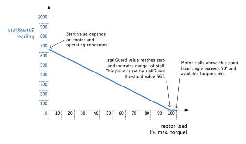
Figure 15.1 Function principle of StallGuard2
