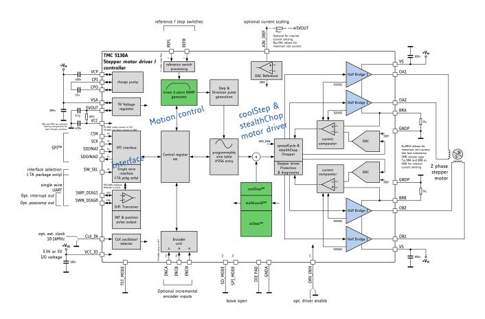
Figure 1.1 TMC5130A basic application block diagram with motion controller
