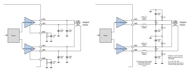
Figure 3.10 Simple ESD enhancement and more elaborate motor output protection
