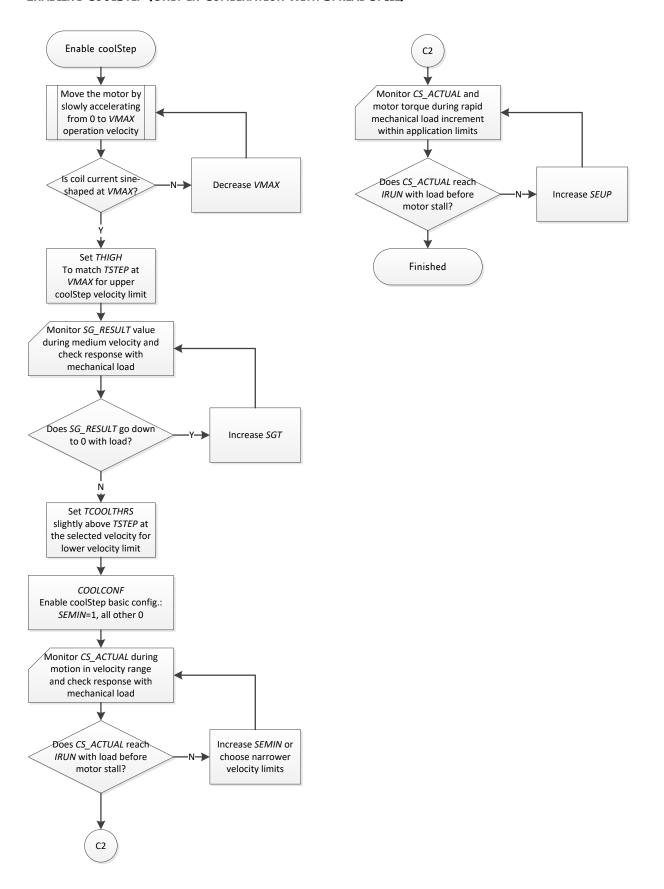
Figure 24.4 Enabling CoolStep (only in combination with SpreadCycle)
