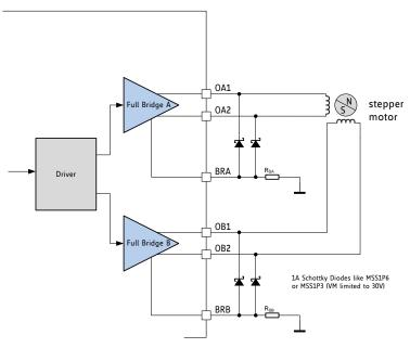
Figure 3.9 Schottky diodes reduce power dissipation at high peak currents up to 2A (2.5A)
