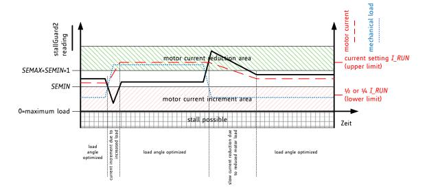
Figure 16.1 CoolStep adapts motor current to the load
