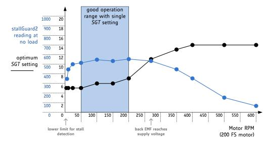
Figure 15.2 Example: optimum SGT setting and StallGuard2 reading with an example motor
