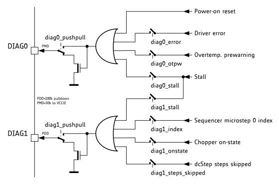
Figure 18.1 DIAG outputs in STEP/DIR mode
