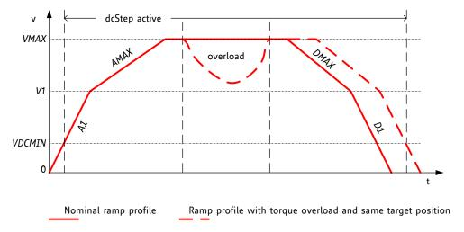
Figure 19.2 Velocity profile with impact by overload situation
