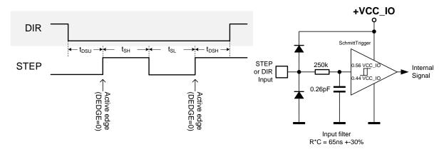
Figure 17.1 STEP and DIR timing, Input pin filter
