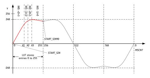
Figure 20.1 LUT programming example
