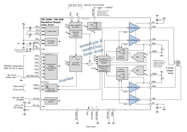
Figure 1.3 TMC5130A standalone driver application diagram
