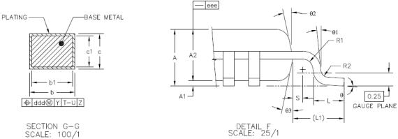
Figure 32.1 Dimensional drawings TQFP48-EP
