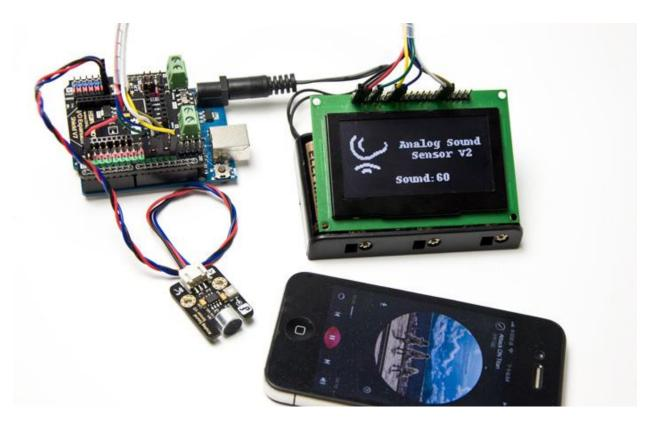
To ease the difficult of using this analog sound sensor, a <u>Gravity</u> Interface is adapted to allow plug&play. The <u>IO expansion shield</u> is the best match for this sound senor connecting to your <u>Arduino</u>. As this sound sensor can work at 3.3V which make it compatible with <u>Raspberry Pi</u>, <u>intel edison</u>, joule and curie.
