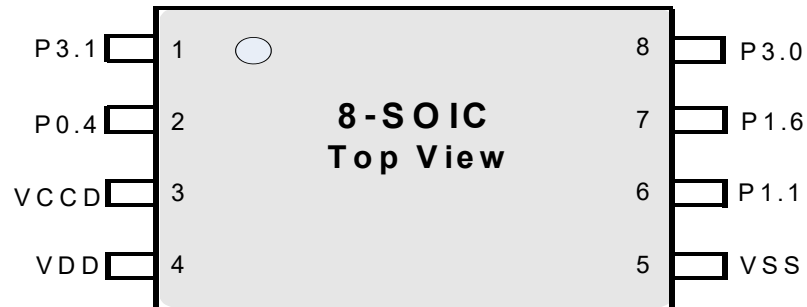
Figure 8. 8-Pin SOIC Pinout
