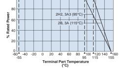
For resistors operated terminal temperature of described for each size or above, a power rating shall be derated in accordance with the derating curve above.
