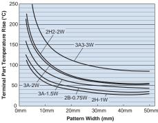
Room Temperature 25°C PCB: FR-4 t=1.6mm Cu foil thickness=35µm While using under high power, the temperature of the product may increase depending on the condition of heat dissipation from PCB. Be sure to check the terminal part temperature as well as precautions for use on delivery specifications before use.
