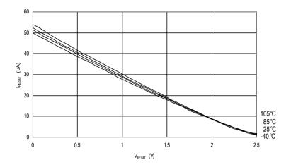
Figure 30-20. Reset Pull-up Resistor Current vs. Reset Pin Voltage (V<sub>CC</sub> = 5V)
