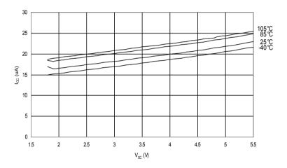
Figure 30-43. Programming Current vs.  $V_{CC}$
