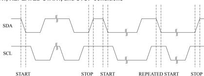
Figure 23-3. START, REPEATED START, and STOP conditions
