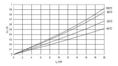
Figure 30-22. I/O Pin Output Voltage vs. Sink Current (V<sub>CC</sub> = 5V)
