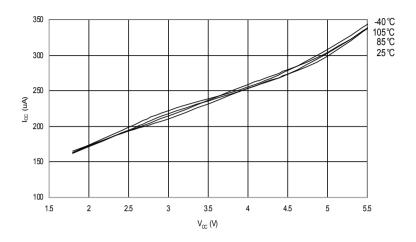
Figure 30-40. Analog Comparator Current vs. V<sub>CC</sub>
