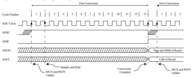
Figure 25-6. ADC Timing Diagram, Auto Triggered Conversion
