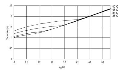
Figure 30-29. Reset Pin Input Threshold vs. V<sub>CC</sub> (V<sub>IL</sub>, I/O Pin Read as '0')
