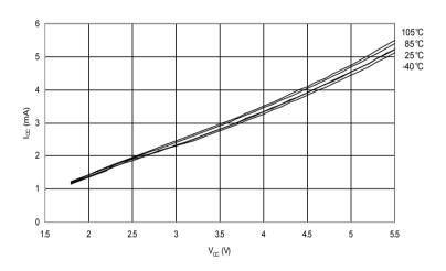
Figure 30-4. Active Supply Current vs. V<sub>CC</sub> (Internal RC Oscillator, 1 MHz)
