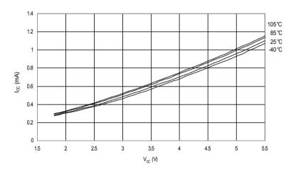
Figure 30-9. Idle Supply Current vs. V<sub>CC</sub> (Internal RC Oscillator, 1 MHz)
