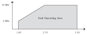
Figure 29-2. Maximum Frequency vs. V<sub>CC</sub>, ATmega164P
