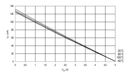
Figure 30-18. Reset Pull-up Resistor Current vs. Reset Pin Voltage (V<sub>CC</sub> = 1.8V)
