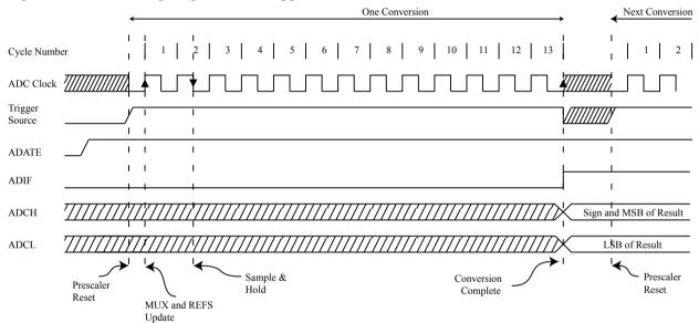
Figure 25-7. ADC Timing Diagram, Free Running Conversion
