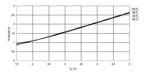
Figure 30-26. I/O Pin Input Threshold vs. V<sub>CC</sub> (V<sub>IL</sub>, I/O Pin Read as '0')
