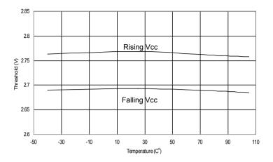
Figure 30-33. BOD Threshold vs. Temperature ( $V_{CC} = 1.8V$ )
