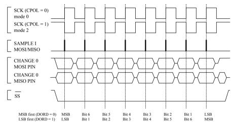
Figure 20-4. SPI Transfer Format with CPHA = 1
