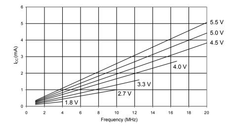
Figure 30-8. Idle Supply Current vs. V<sub>CC</sub> (Internal RC Oscillator, 8 MHz)
