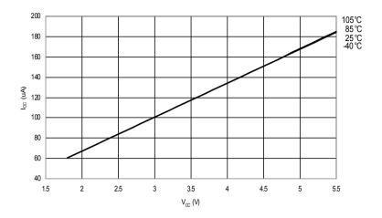
Figure 30-42. Brownout Detector Current vs. V<sub>CC</sub>
