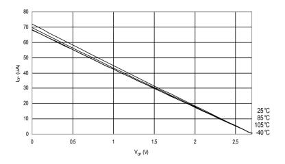
Figure 30-17. I/O Pin Pull-up Resistor Current vs. Input Voltage (V<sub>CC</sub> = 5V)
