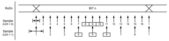
The decision of the logic level of the received bit is taken by doing a majority voting of the logic value to the three samples in the center of the received bit: If two or all three center samples (those marked by
