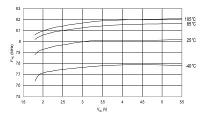
Figure 30-37. Calibrated 8MHz RC Oscillator vs. Temperature
