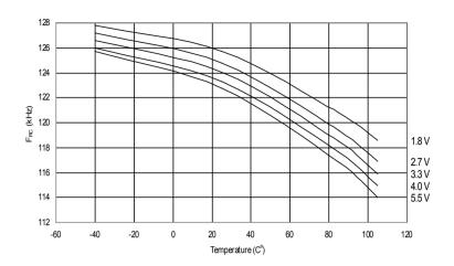
Figure 30-35. Watchdog Oscillator Frequency vs. V<sub>CC</sub>
