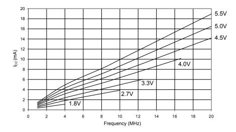
Figure 30-3. Active Supply Current vs. V<sub>CC</sub> (Internal RC Oscillator, 8 MHz)
