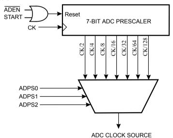
By default, the successive approximation circuitry requires an input clock frequency between 50kHz and 200kHz to get maximum resolution. If a lower resolution than 10 bits is needed, the input clock frequency to the ADC can be higher than 200kHz to get a higher sample rate.
