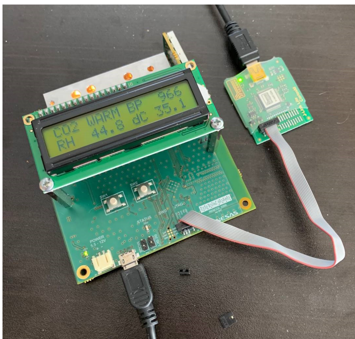
Figure 14. RTD120D-EVK Evaluation Kit with Debugger
