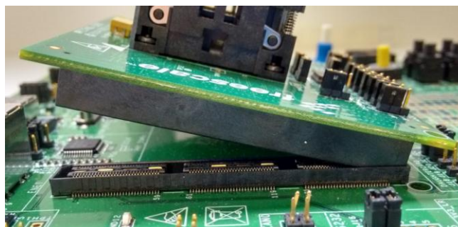
Figure 3. Removing a daughtercard
