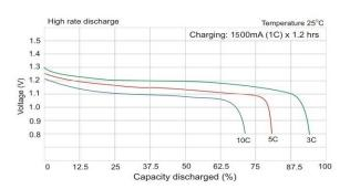
The data shown is correct at a temperature of 20±5°C Shutdown at-ΔV= 15mV, after reaching 120% of the rated capacity or at a temperature above 55°C
