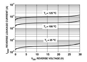
Figure 28. SyncFET<sup>™</sup> Body Diode Reverse Leakage vs. Drain-Source Voltage
