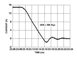
Figure 27. FDMS7608S SyncFET<sup>™</sup> Body Diode Reverse Recovery Characteristic
