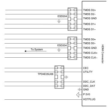
Figure 11. ESD204 Protecting the HDMI Interface
