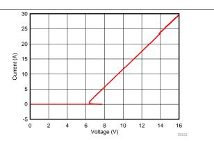
Figure 2. Negative TLP Curve, GND to IO pin (t<sub>p</sub>=100 ns; Plotted as Positive TLP Curve from GND to IO pin)
