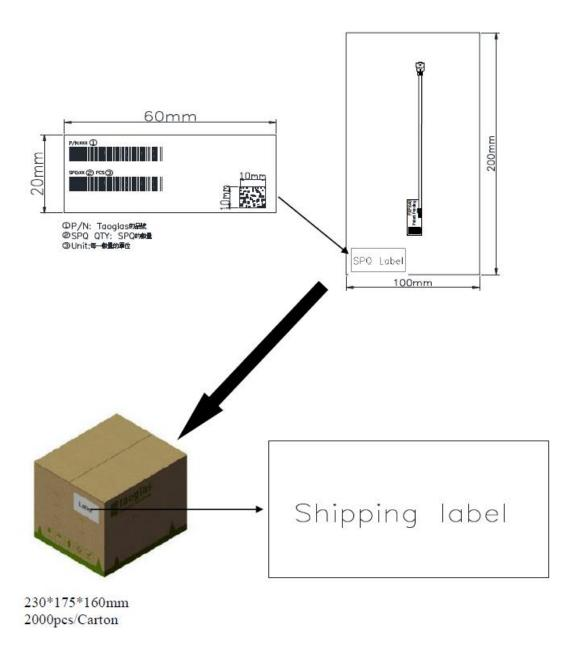
Figure 16. Package of the FXP840 Antenna.
