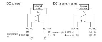
NO Note: Leakage current from indicator circuit may cause load's malfunction. Please check the load's OFF current before use the indicator-equipped switch.
