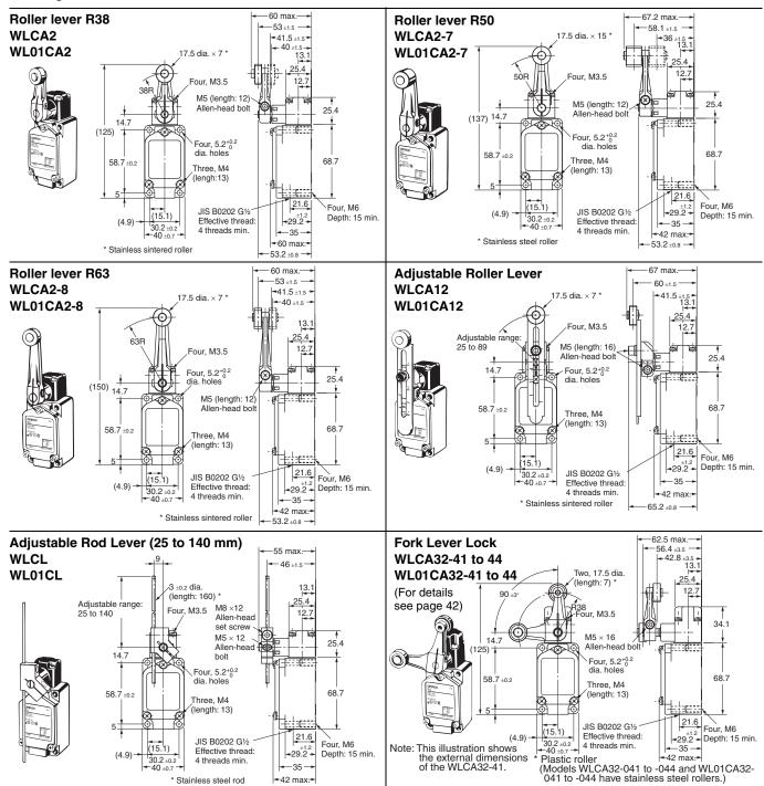
Note: Unless otherwise indicated, a tolerance of  $\pm 0.4 \ \text{mm}$  applies to all dimensions.
