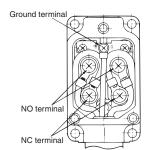
The ground terminal is only installed on models with ground terminals.
