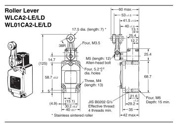
Note: Unless otherwise indicated, a tolerance of  $\pm 0.4 \ \text{mm}$  applies to all dimensions.
