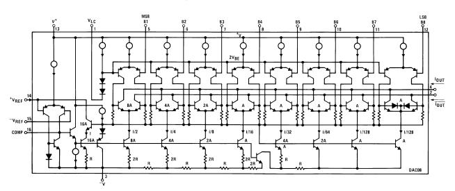
Figure 17. Equivalent Circuit
