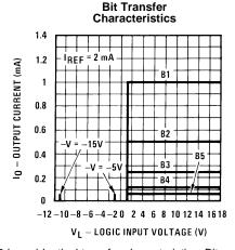
Note. B1–B8 have identical transfer characteristics. Bits are fully switched with less than ½ LSB error, at less than  $\pm 100$  mV from actual threshold. These switching points are guaranteed to lie between 0.8 and 2V over the operating temperature range ( $V_{LC} = 0V$ ). Figure 13.
