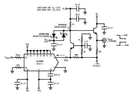
Figure 29. Settling Time Measurement
