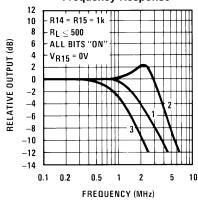
Curve 1:  $C_C$ =15 pF,  $V_{IN}$ =2 Vp-p centered at 1V. Curve 2:  $C_C$ =15 pF,  $V_{IN}$ =50 mVp-p centered at 200 mV. Curve 3:  $C_C$ =0 pF,  $V_{IN}$ =100 mVp-p centered at 0V and applied through 50Ω connected to pin 14.2V applied to R14. Figure 7.
