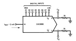
Pin numbers represent the PDIP package. The SOIC package pin numbers differ from that of the PDIP package.
