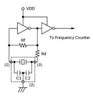
Regarding CERALOCK® with built-in capacitors, the terminal (1) and (3) are interchangeable, but if connection is interchanged, the specification of initial tolerance frequency may not be guaranteed. \*Please see dimensions about terminal numbers.
