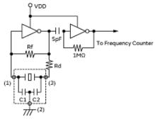
Regarding CERALOCK® with built-in capacitors, the terminal (1) and (3) are interchangeable, but if connection is interchanged, the specification of initial tolerance frequency may not be guaranteed. \*Please see dimensions about terminal numbers.
