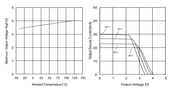
Figure 34. Maximum Output Voltage (High) vs Ambient Temperature ( $V_{CC}$ =5V,  $R_L$ =2 $k\Omega$ )
