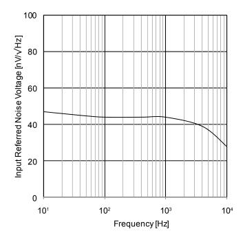
Figure 52. Input Referred Noise Voltage vs Frequency ( $V_{\text{CC}}$ =5V)
