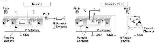
Figure 68. Example of monolithic IC structure
