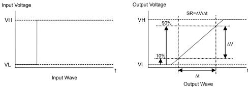
Figure 61. Slew Rate Input and Output Wave
