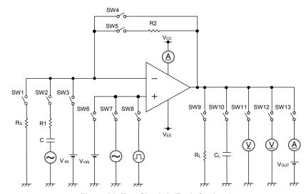
Figure 60. Test Circuit 2 (Each Op-Amp)
