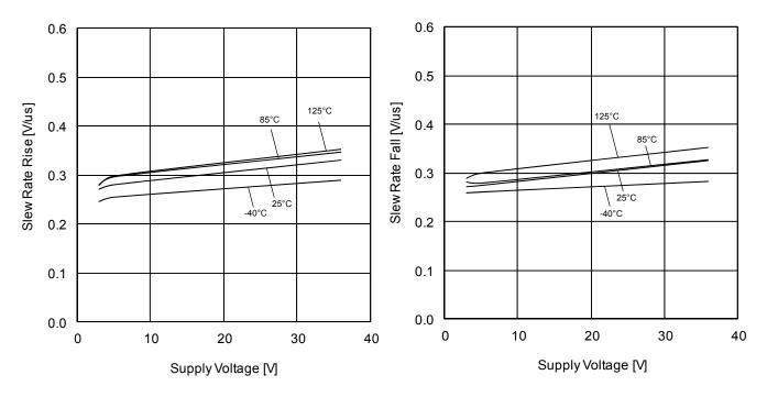
Figure 21. Slew Rate Rise vs Supply Voltage ( $R_L$ =2 $k\Omega$ , Low to High)
