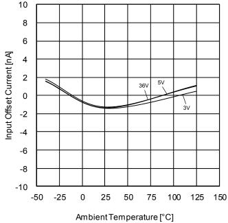
Figure 48. Input Offset Current vs Supply Voltage (V<sub>ICM</sub>=V<sub>CC</sub>/2, E<sub>K</sub>=-V<sub>CC</sub>/2)
