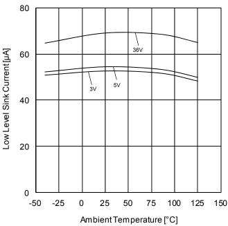
Figure 41. Low Level Sink Current vs Ambient Temperature (V<sub>OUT</sub>=200mV)
