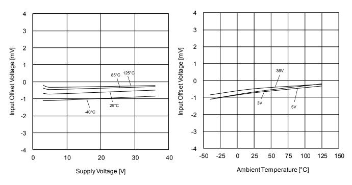
Figure 42. Input Offset Voltage vs Supply Voltage (V<sub>ICM</sub>=V<sub>CC</sub>/2, E<sub>K</sub>=-V<sub>CC</sub>/2)
