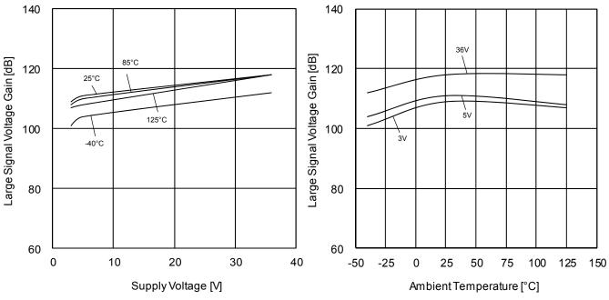
Figure 54. Large Signal Voltage Gain vs Supply Voltage (R<sub>L</sub>=2kΩ)
