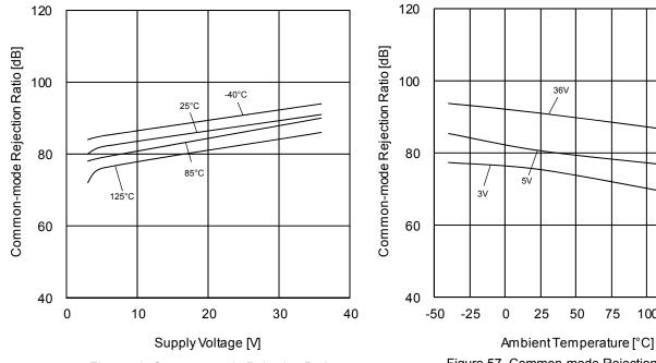
Figure 56. Common-mode Rejection Ratio vs Supply Voltage
