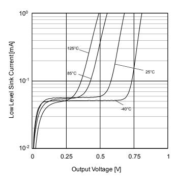
Figure 11. Low Level Sink Current vs Output Voltage (Enlarged view)  $(V_{CC}=5V)$
