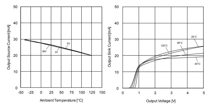
Figure 7. Output Source Current vs Ambient Temperature (V<sub>OUT</sub>=0V)
