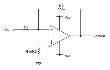
Figure 65. Inverting Amplifier Circuit
