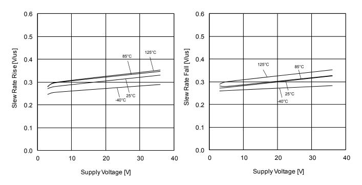
Figure 50. Slew Rate Rise vs Supply Voltage ( $R_L$ =2 $k\Omega$ , Low to High)
