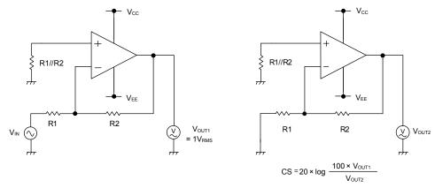
Figure 62. Test Circuit 3 (Channel Separation)  $(R1 {=} 1k\Omega, R2 {=} 100k\Omega)$
