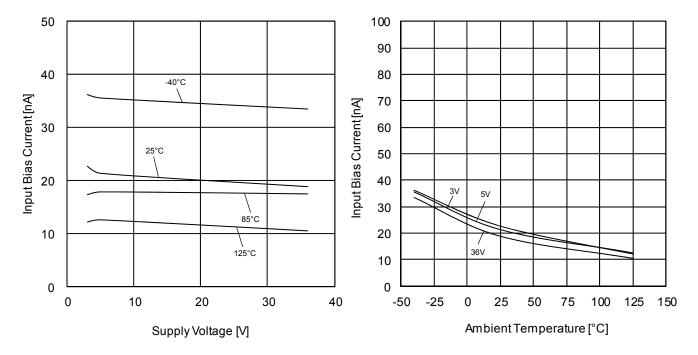
Figure 44. Input Bias Current vs Supply Voltage (V<sub>ICM</sub>=V<sub>CC</sub>/2, E<sub>K</sub>=-V<sub>CC</sub>/2)
