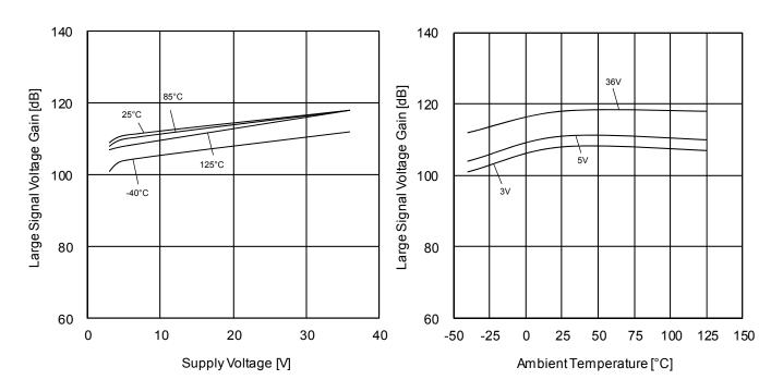
Figure 25. Large Signal Voltage Gain vs Supply Voltage ( $R_L$ = $2k\Omega$ )
