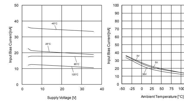
Figure 15. Input Bias Current vs Supply Voltage (V<sub>ICM</sub>=V<sub>CC</sub>/2, E<sub>K</sub>=-V<sub>CC</sub>/2)
