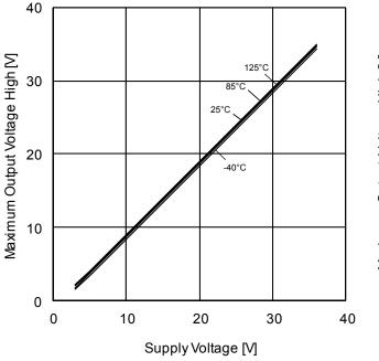
Figure 3. Maximum Output Voltage (High) vs Supply Voltage ( $R_L$ =10k $\Omega$ )
