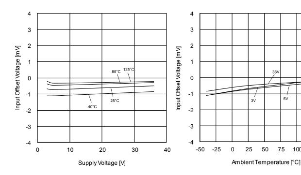
Figure 13. Input Offset Voltage vs Supply Voltage (V<sub>ICM</sub>=V<sub>CC</sub>/2, E<sub>K</sub>=-V<sub>CC</sub>/2)
