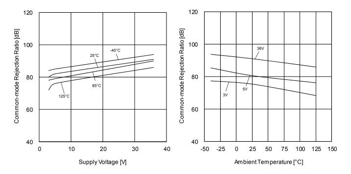
Figure 27. Common-mode Rejection Ratio vs Supply Voltage
