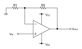
Figure 66. Non-inverting Amplifier Circuit
