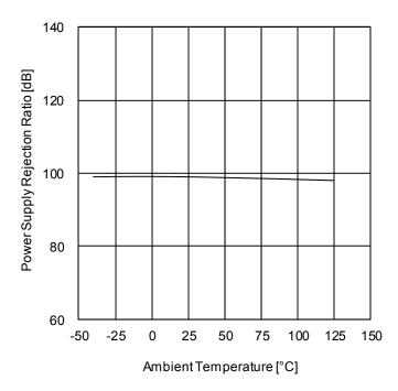
Figure 29. Power Supply Rejection Ratio vs Ambient Temperature
