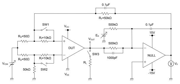
Figure 59. Test Circuit 1 (One Channel Only)
