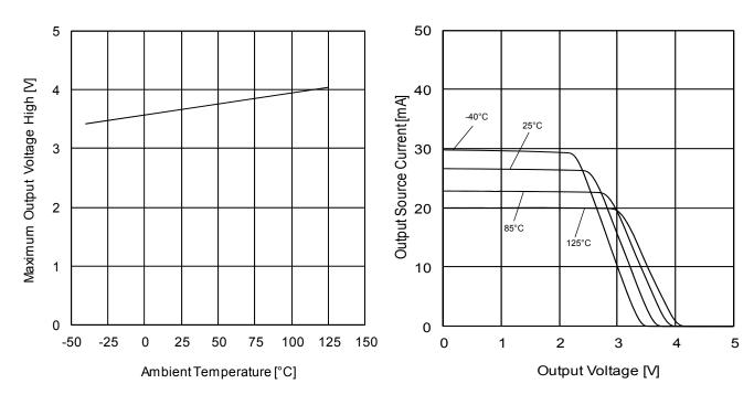
Figure 5. Maximum Output Voltage (High) vs Ambient Temperature ( $V_{CC}$ =5V,  $R_L$ =2 $k\Omega$ )
