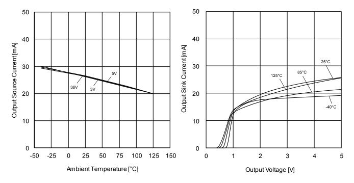
Figure 36. Output Source Current vs Ambient Temperature (Vout=0V)
