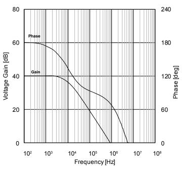
Figure 53. Voltage Gain, Phase vs Frequency (V<sub>CC</sub>=30V, R<sub>L</sub>=2k $\Omega$ , C<sub>L</sub>=100pF)
