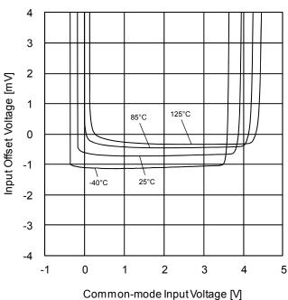
Figure 18. Input Offset Voltage vs Common-mode Input Voltage (V<sub>CC</sub>=5V)
